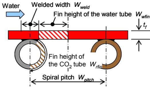
Fig.5 Analysis model of fin efficiency
