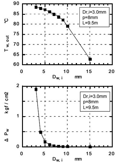
Fig.7 Influence of water tube diameter
