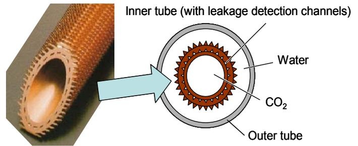
Fig.2 Double tube HX with leakage detection channels
