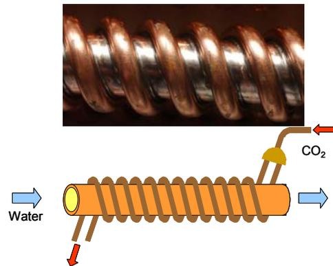
Fig.3 Photo and Schematic view of the developed HX
