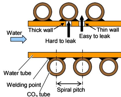
Fig.4 Leakage detection mechanism
