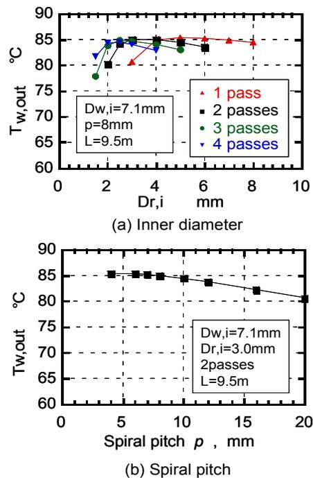
Fig.8 Influence of specification of CO<sub>2</sub> tube
